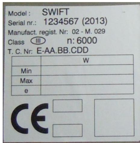
Figure 1.4.1 Label with characteristics and metrological identification layout
